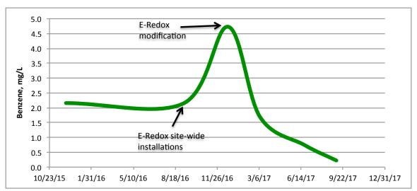
Overall benzene concentrations for the source area of a fuel station. Around November 2016 groundwater level onsite dropped significantly, corresponding to the increase of benzene level at the source area.
