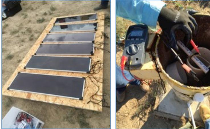
**Figure 7. Solar panels as power source for E-Redox<sup>®</sup> pilot system, and monitoring of electrical parameters**
